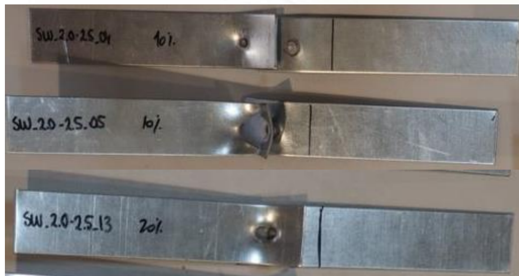
Spot welds loaded in shear
